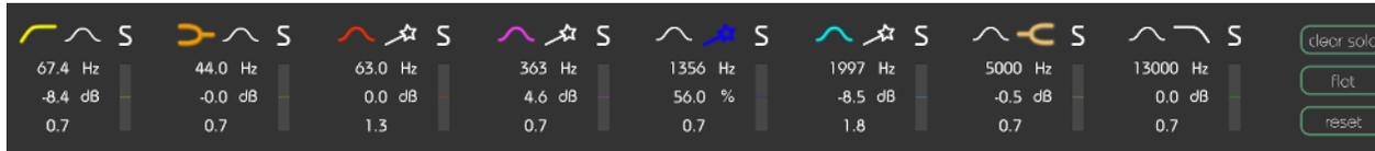
The parameter section shows eight filter bands and their related parameters. When hovering over the parameter section of a band, the band is highlighted with the color of the related filter curve inside the interactive EQ display. Hovering over a band with a smart filter (wand symbol), the related smoothing slider in the master section will be highlighted as well.
