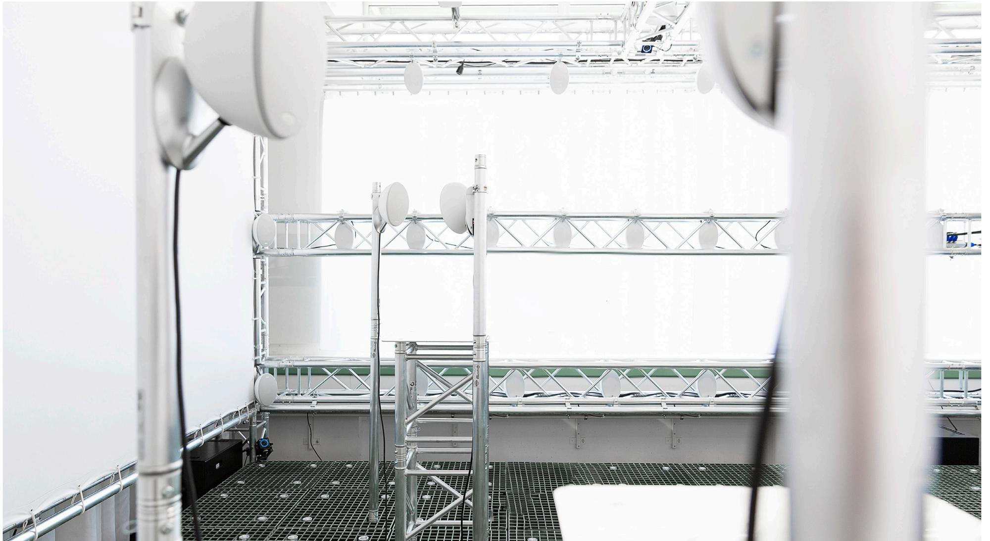
Each of **sonible's six d:24s** combines an analog to digital converter and an amplifier. This makes **additional devices** in the signal chain **unnecessary**.
