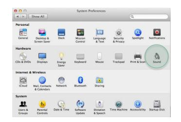
In the Sound menu, navigate to the Output tab and select the device called sonible ml:1 as output device.
