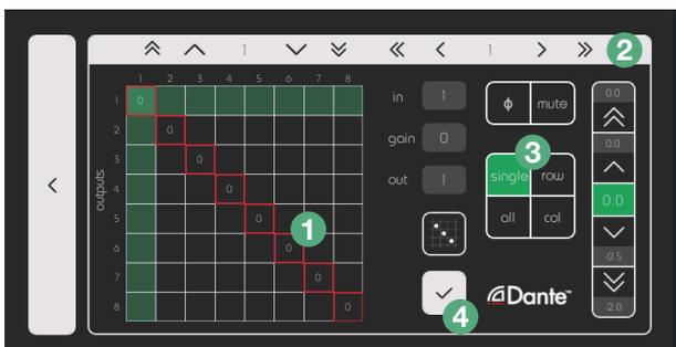
In the routing menu you are able to route the inputs to the outputs, modify settings such as gain reduction, phase inversion and to mute a selected input channel.
