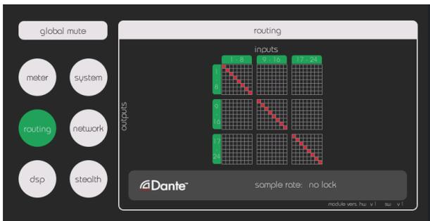
At firmware versions higher than 3.0 the routing screen displays a matrix.
