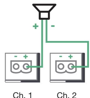
**NOTE: Please be VERY careful when bridging channels! Incorrect wiring can damage the corresponding amplifier channels as well as the connected speaker. The bridged loudspeaker may not be connected to the ground under no circumstances.**
