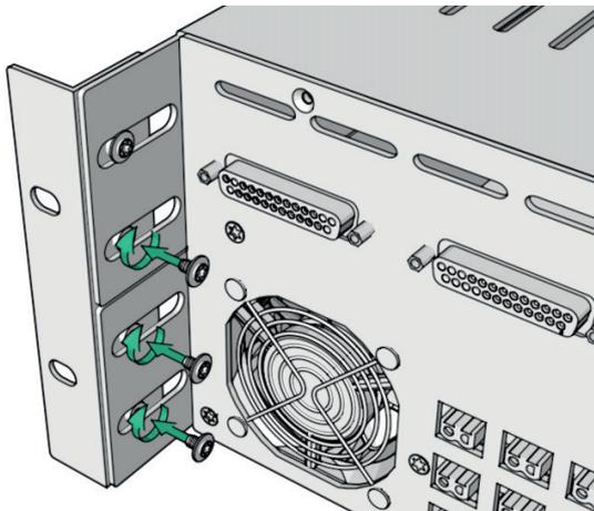
The amplifier is three rack units high (3RU) and fits into a standard EIA 19" rack or cabinet. The depth of the amplifier is 517mm (20,4"). The weight of the analog version is approximately 20 kg (44 lbs).
