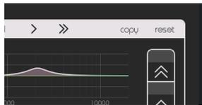
The copy-paste function is available on the top right at any time in the dsp channel menu. Use it to copy the settings of the selected channel.
