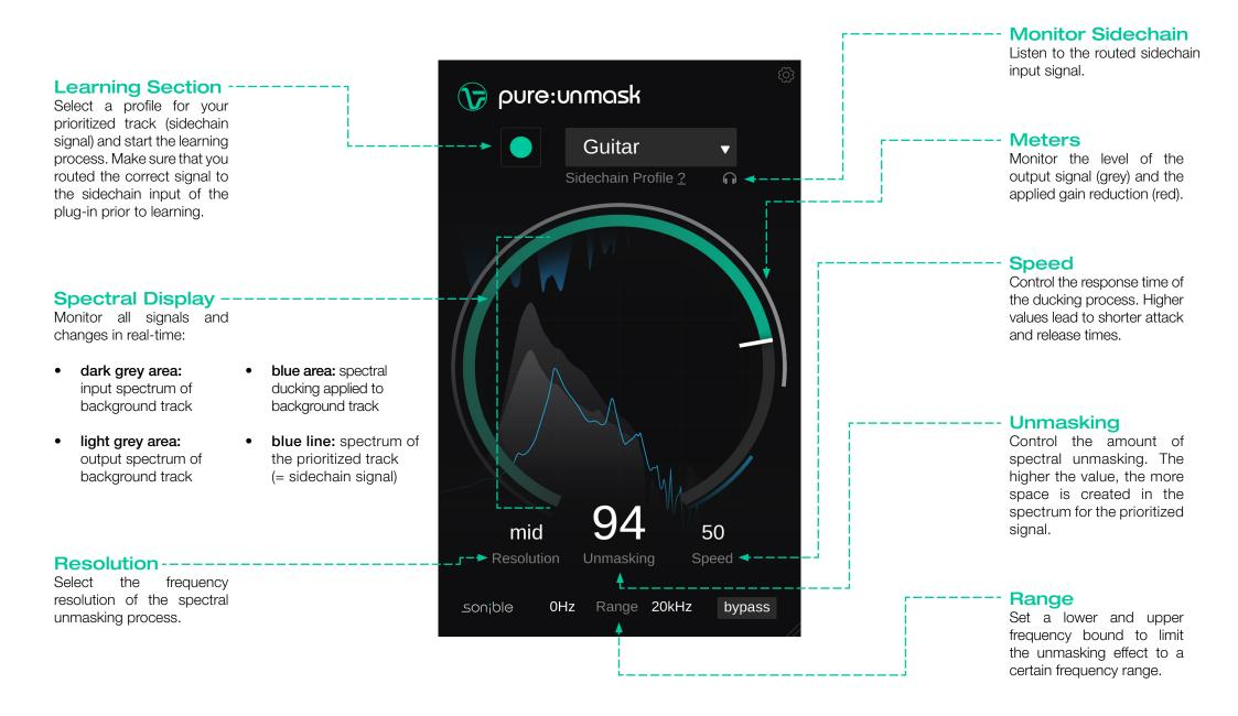
pure:unmask creates space for a prioritized track by dynamically ducking frequencies in a background track that cause cluttering. Common scenarios are e.g. a vocal competing with a piano track or a kick drum overlapping with a bass.
